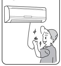
When cleaning, power supply must be disconnected.
