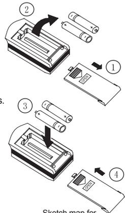
Sketch map for replacing batteries
