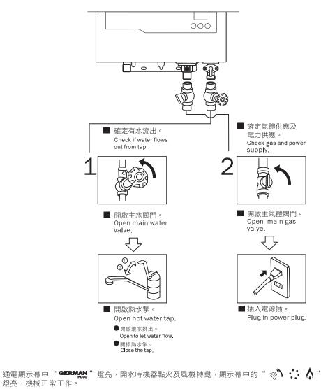
After connecting to power supply, the "GERMAN" logo on the display will light up. Turn on the water supply, the heater ignition and fan will start at same time, then the "
